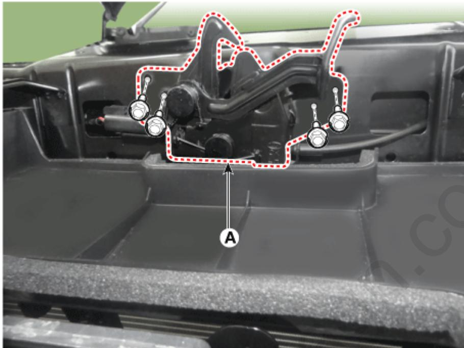
3. Disconnect the hood latch cable (A).
